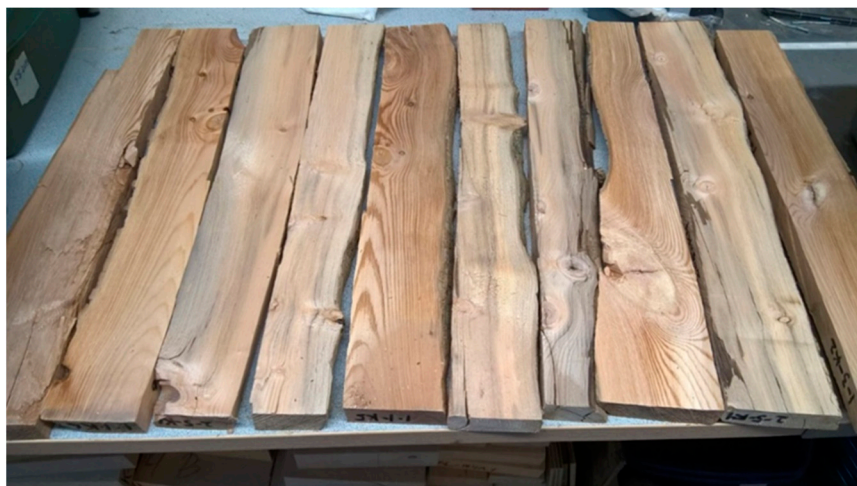
Figure 2. A set of unedged subfossil Scots pine boards prepared for the manufacturing of a physico-mechanical test specimen.
