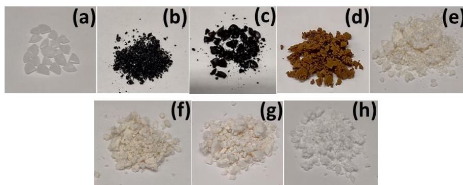
Figure 4. Recovered materials after treatment of in PVDF in [EMIM][AcO] IL, AA and DESs with varying AA:IL mole ratios, (a) neat PVDF, thermally treated PVDF in (b) pure IL, (c) AA:IL = 1:1, (d) AA:IL = 2:1, (e) AA:IL = 3:1, (f) AA:IL = 4:1, (g) AA:IL = 6:1 and, (h) pure AA. Temperature = 140 °C, time = 1 h.
