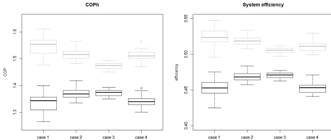
Figure 9. The coefficient of performance is defined as heat used to generated steam divided by the main motor consumption (i.e.  $COP_h = Q_s/W$ ). The system efficiency is defined as the measured  $COP_h$  divided by the Carnot COP (i.e.  $\eta_{system} = COP_h/COP_{carnot}$ ). The box and whisker plots in grey are estimated values for a fully thermally insulated heat pump.
