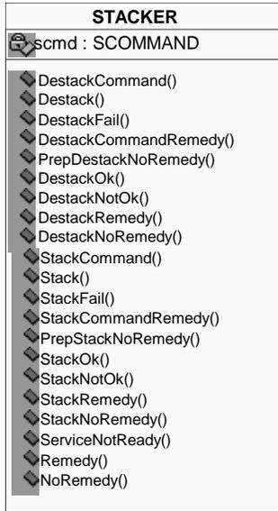
Figure 5. Specification class diagram for the Stacker unit.
