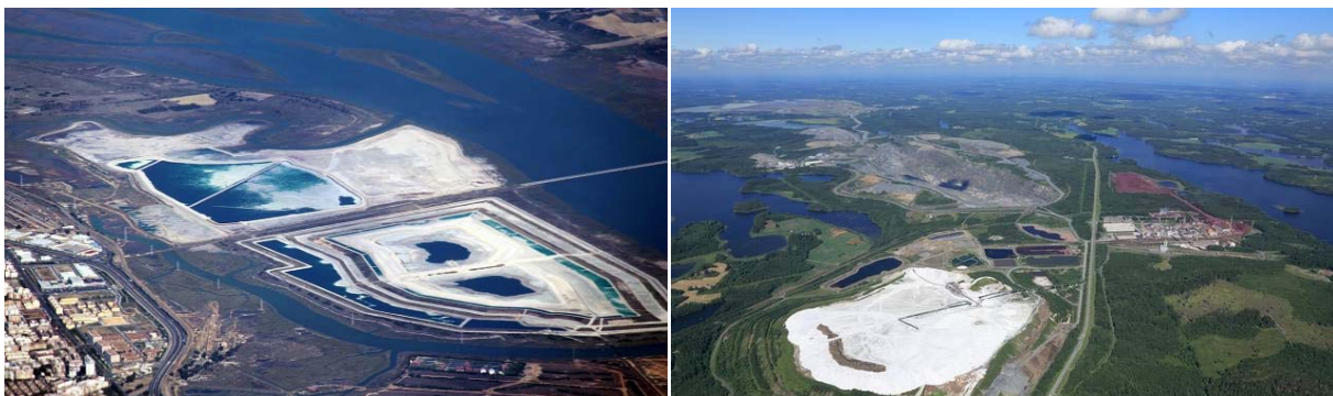
Figure 1: Deposits of phosphogypsum: at Huelva, Spain, covering \sim 1200 ha (left) 1 and near Siilinjärvi, Finland, covering \sim 60 ha (right) 2
