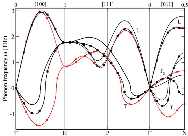
FIG. 1. (Color online) Phonon dispersions for  $\gamma$ -U at 500 K. SCAILD coupled with FPLMTO without spin-orbit interaction (black line solid squares), with SO (black solid line), and with VASP-PAW (red line solid circles).
