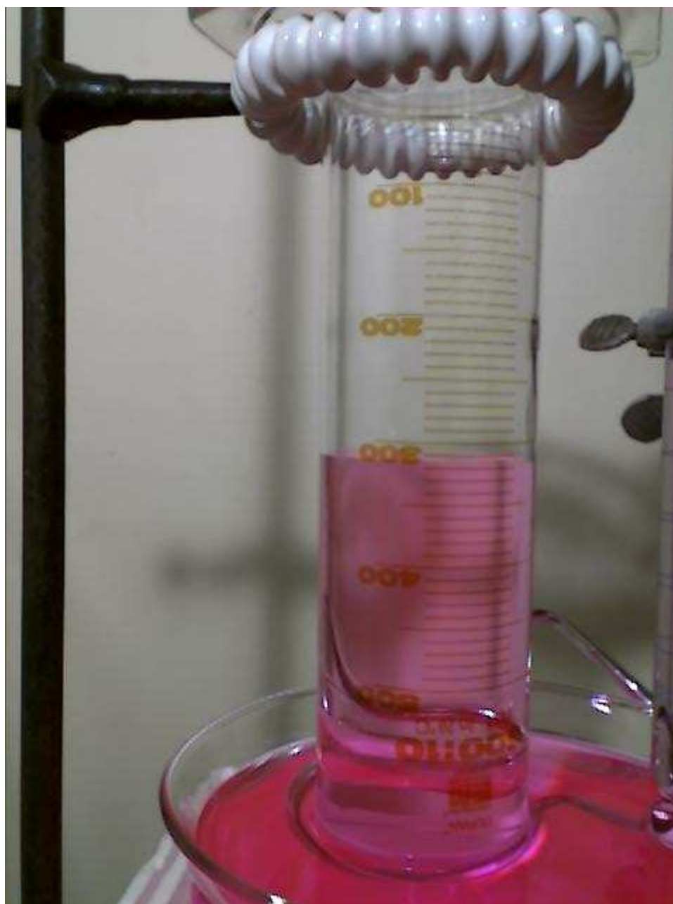
Figure 1. The setup. The dyed water rises slowly inside the graduated cylinder as the \text{CO}_2 atmosphere inside the cylinder dissolves into the water. The image is one of the \sim 6000 recorded during the course of the experiment.
