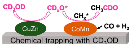
Figure 2. Proposed reaction mechanism for formation of alkanal based on in situ DRIFTS-MS results. Reproduced from ref. [49] Copyright (2021) with permission from ACS publications.
