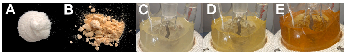
Fig. 4. Yellowing effect of iodate-contaminated microcrystalline cellulose at room temperature (A), after drying in the oven for 24 h at 80 °C (B), iodate-contaminated solubilized dialdehyde cellulose at 100 °C after heating for 35 min (C), 45 min (D), and 80 min (E).
