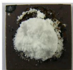
Fig. 11. a) Average corrosion rates (mm/year) of carbon steel (P235GH) after exposure at 80 °C to different calcium salts mixtures. The tests were performed at various water contents in the gas (15, 20, and 25 vol%) for 72 h. b) Pictures of the three salt mixtures taken a few minutes after the exposure at 25 vol% H 2 O. A semi-wet solution had formed in the two deposits comprising 5 and 25 wt% CaCl 2 due to the lower amount of deliquescent CaCl 2 in the mixture.
