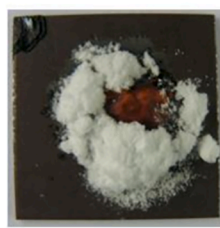
Fig. 11. a) Average corrosion rates (mm/year) of carbon steel (P235GH) after exposure at 80 °C to different calcium salts mixtures. The tests were performed at various water contents in the gas (15, 20, and 25 vol%) for 72 h. b) Pictures of the three salt mixtures taken a few minutes after the exposure at 25 vol% H 2 O. A semi-wet solution had formed in the two deposits comprising 5 and 25 wt% CaCl 2 due to the lower amount of deliquescent CaCl 2 in the mixture.
