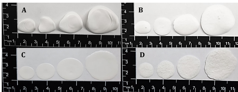
Figure 8. Semi-solid extrusion (SSE)-based 3D-printed films containing nanoparticles of piroxicam. Films printed with printing ink 1 and (A) dried at room temperature and (B) freeze-dried. Films printed with printing ink 2, (C) dried at room temperature, and (D) freeze-dried. Reproduced from (VI), with permission from Elsevier.
