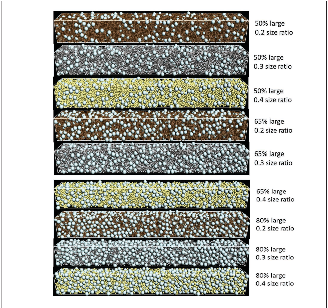
3. Examples of bimodal packing of spheres in a three-dimensional geometry for various size ratios and volume concentrations of large particles.
