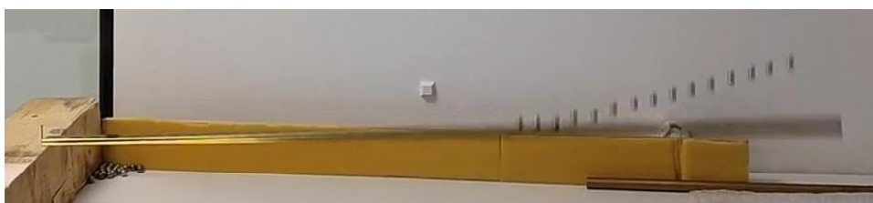
Figure 6. The falling rod loaded with 15 steel beads as it reaches the horizontal level. Frame extracted from a mobile phone filming at 60 fps the same experiment as in Fig. 3.
