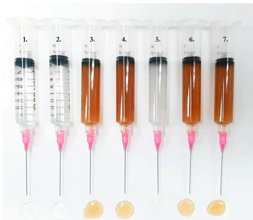
Figure 2. Solution-filled syringes attached with 1.5-inch 20 G precision dispensing tips and their extrudates. (1) Unloaded solution, (2) drug-loaded solution, (3) unloaded solution with liver powder, (4) drug-loaded solution with liver powder, (5) 2% drug-loaded solution, (6) nonprintable unloaded solution, and (7) nonprintable drug-loaded solution.
