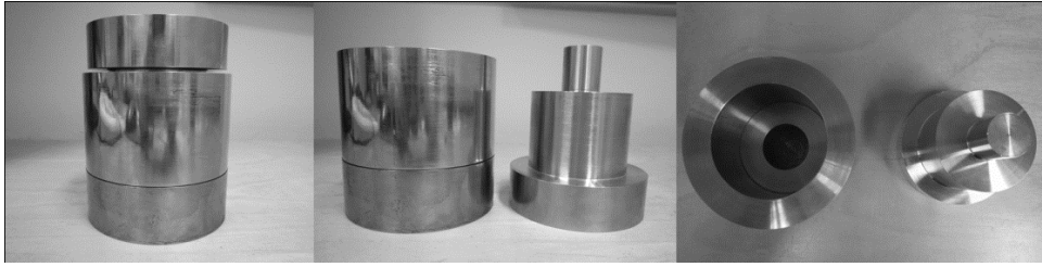
Fig. 2 Pictures of prototype mould from stainless steel
